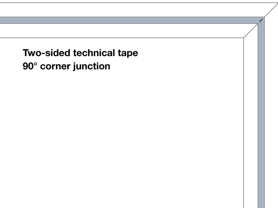
Polycarbonate 90° corner profile
