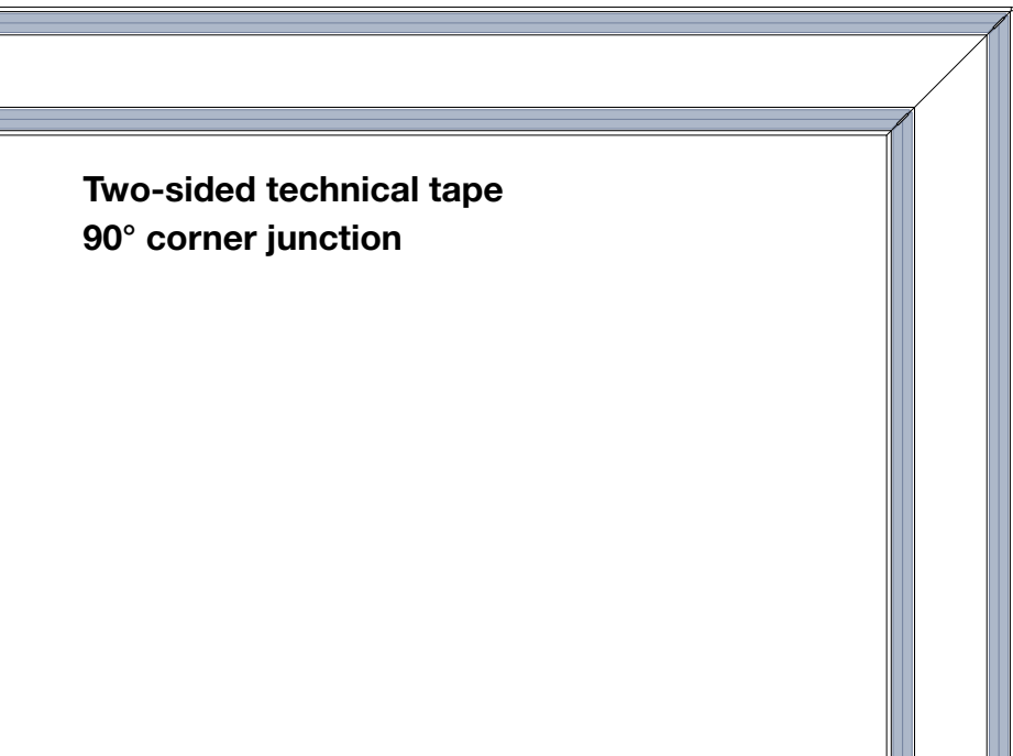
Polycarbonate 90° corner profile
