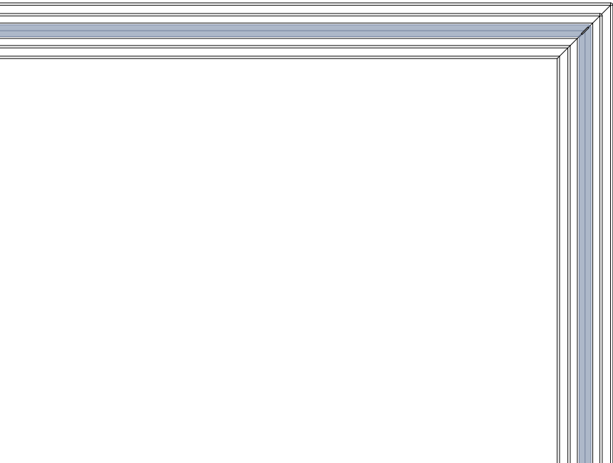
Two-sided technical tape 90° corner junction
